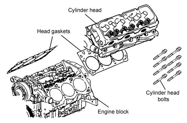
\*Note that the second cylinder head and its bolts are not shown in this image
